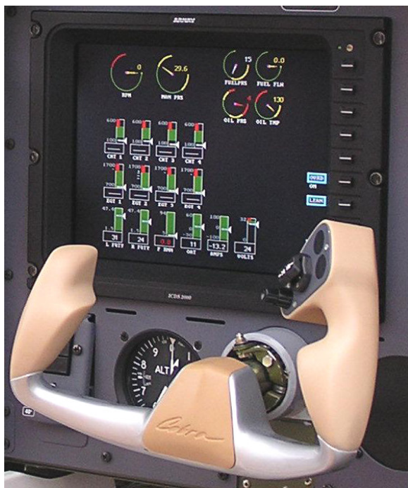
Fig 9. Software interface: graphical presentation of engine/systems data (VUT 100 Cobra airplane)
