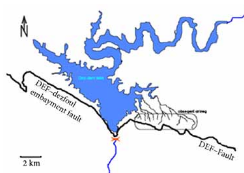
Fig. 6. Obsequent structure of drainage network due to of DEF function in the Dez Dam
