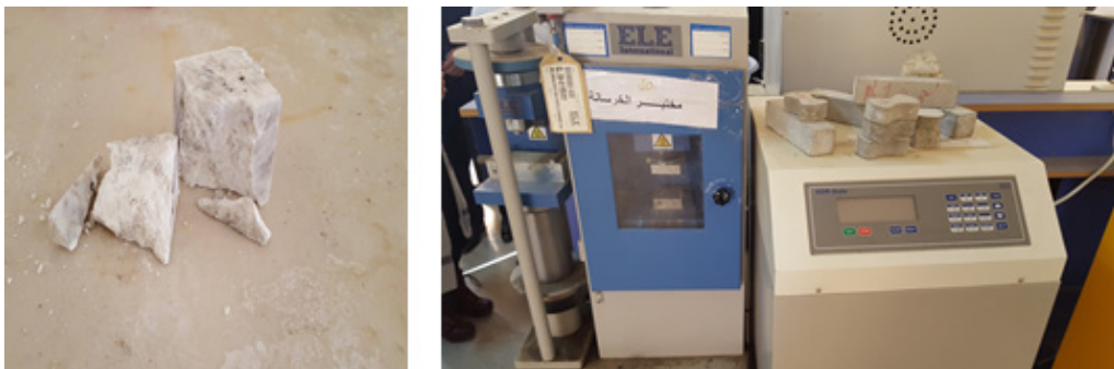
Figure 7. Sample cube assay in compression device and test result
