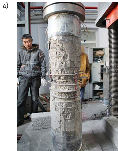
Figure 6. Failure pattern of confined concrete: a) bulging: ACS-Y-9; b) shear sliding: ACS-Y-8
