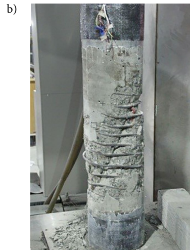
Figure 6. Failure pattern of confined concrete: a) bulging: ACS-Y-9; b) shear sliding: ACS-Y-8
