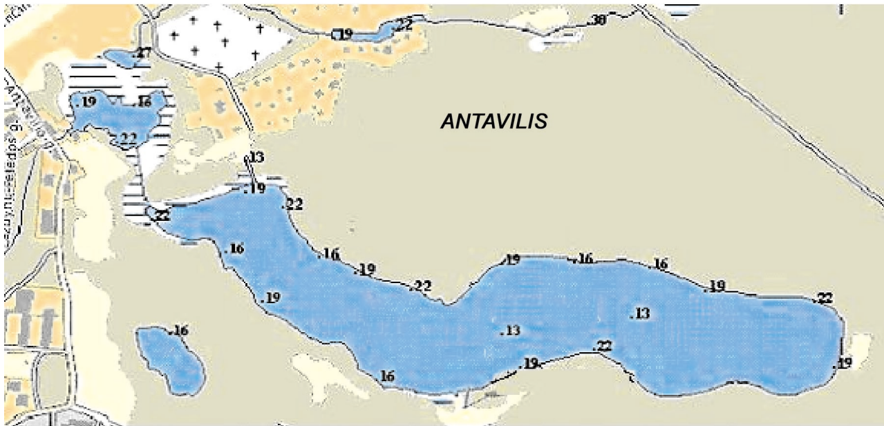
Fig 3. Water reservoirs in Antaviliai (each number corresponds to an average value of equivalent dose rate [nSv/h] in an investigated place)
