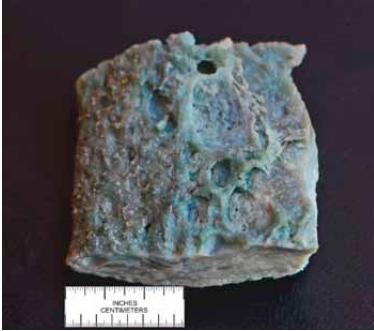
Fig. 3. Deposit formation pattern from the pilot biomass-firing stoker found during the annual maintenance procedure (Photo by A. Baleckis)
